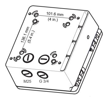
VDA-AD-JNB mounting hole measurements - back/rear
