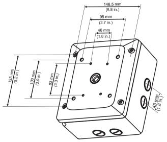
VDA-AD-JNB mounting hole measurements - front
