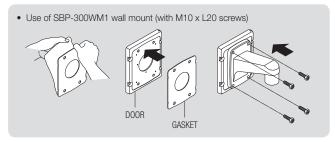
Use of SBP-300WM wall mount (evenly securing the wall mount inside the gasket groove as shown in the image below.) (with M10 x L12 screws)
