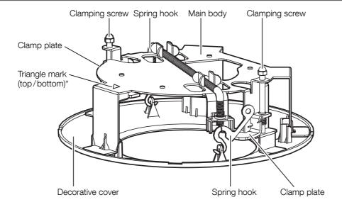
\* Because the triangle mark is engraved on the bracket, it can be seen from both the top and bottom
